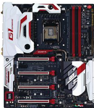
Gigabyte's Z170X-Gaming-G1 motherboard handles Intel's 6th generation Core processors with optional liquid cooling support.
