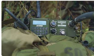
1. The Falcon II AN/PRC-150(C) is a portable HF tactical military radio for voice and data communications from 1.6 to 59.999 MHz.
